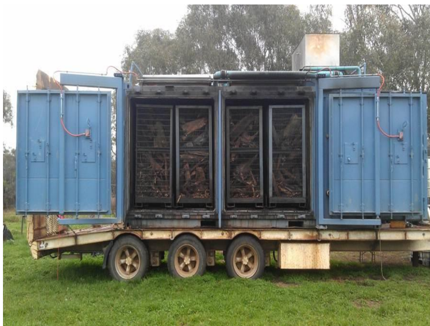
Figure 2. CharMaker commercial facility used for pyrolysing biosolids in this study.
