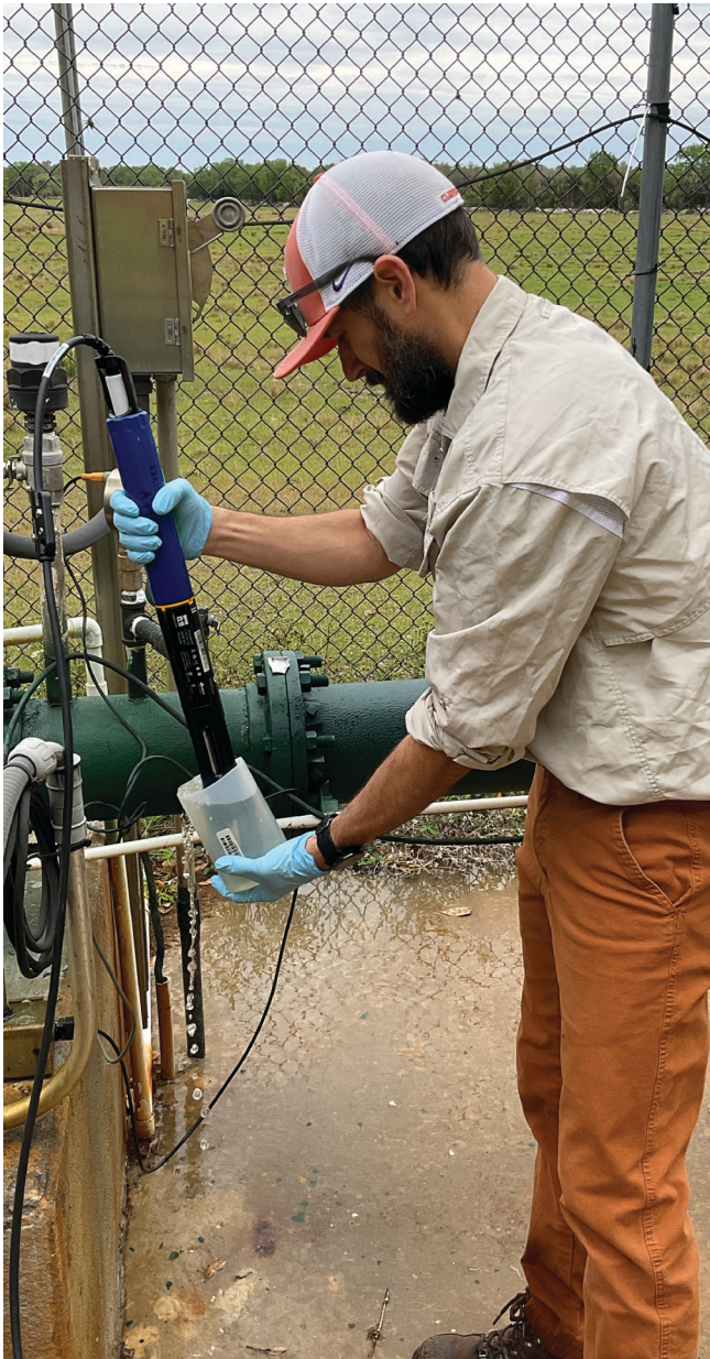
EPA Region 4 environmental engineer Landon Pruitt samples groundwater for PFAS at the Seminole Tribe of Florida's Brighton Reservation.
